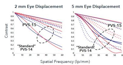
The key metric for the eyepiece is its performance over the eye box, showcasing a performance level commensurate with the PVS-15 (gold standard) over the eye box
