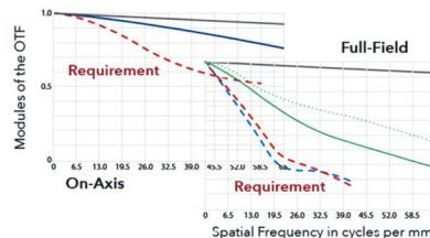
The as-designed and as-manufactured performance surpasses MIL-SPEC requirements across the temperature range.
